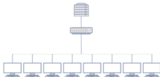
2 LANS topology: Network with 8 clients, 1 router
