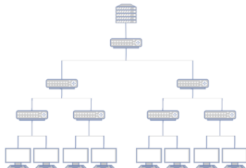
Network with 8 clients 2 clients per LAN, 7 Routers
