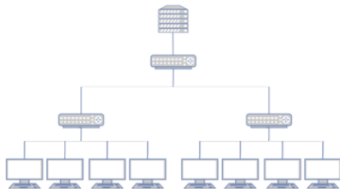
Network with 8 clients 4 clients per LAN, 3 Routers
