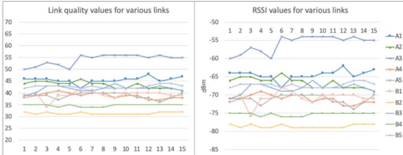
Figure 4. Link quality indicator and RSSI measurements.
