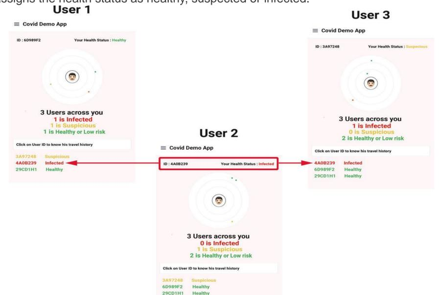
When 3 mobile phones with pre-installed COVID applications and integrated with 3 COVID smart watch were brought in the Bluetooth vicinity of one another, the users were able to see the other BLE devices using the BLE meshnetworking protocol installed within the application.
