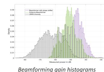
Beamforming gain histograms >15 dB for 50% (antenna + phase shifters)
