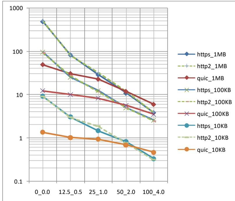
➤ QUIC is affected less by losses and network delays
