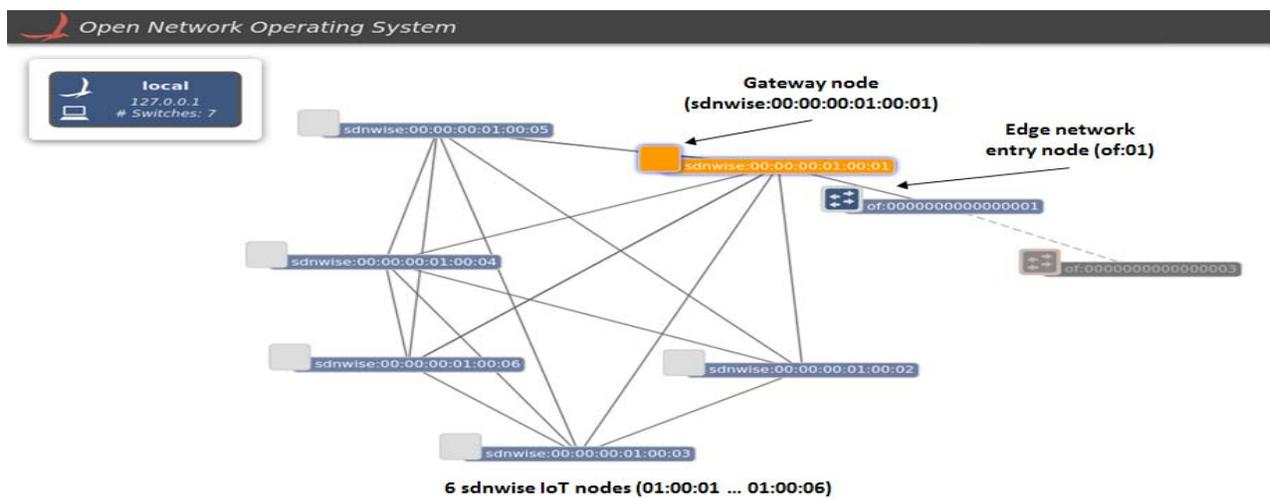
Fig. 4. ONOS snapshot of IoT set-up
