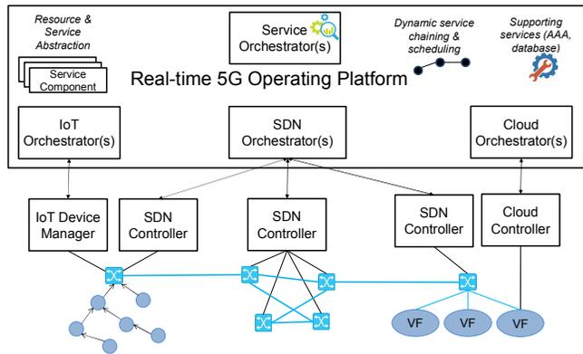
Fig. 2. Reference architecture and building blocks
