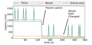
Fig. 3. Latency readings from node 4. First, a parent switch occurs in the 6TiSCH network. Secondly, the wired topology is modified as well to minimize the overall end-to-end latency.
