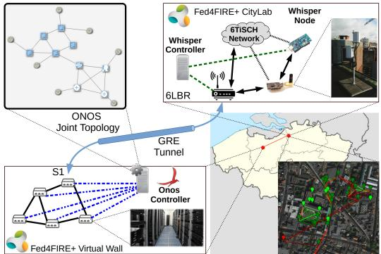
ig. 2. Architecture of the multi-domain network deployed in two different Fed4FIRE+ testbeds to provide end to end control.
