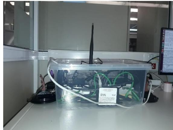
Experiment nodes mounted in vehicles ("SDR-OBUs")
