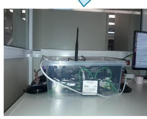
Experiment nodes mounted in vehicles ("SDR-OBUs")
