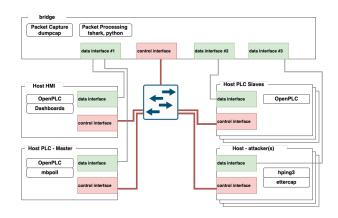
Fig. 1. Overall architecture with PLCs
